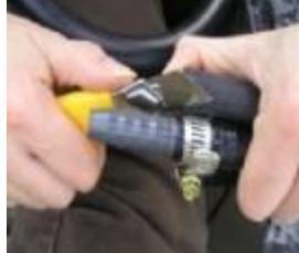
All joints between tubing should be secured tightly with hose clamps. When cutting the tubing to allow the clamp to fit make sure to cut into the keel edge of the tubing. Avoid cutting the airline with the blade. Be careful not to cut yourself!
