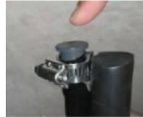
The ends of the tubing should be plugged with a 1/2" PVC or brass plug which has been clamped with a hose clamp. Again, use a blade to cut a small separation between the airline and the solid core keel so your clamp will slide into the airline.
